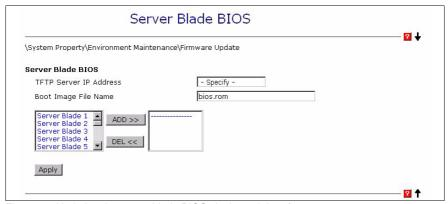
Figure 21: Updating the server blade BIOS via the web interface
